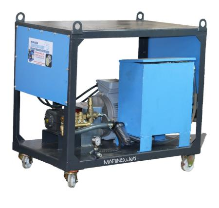
The MR350/21 Water jet Machine is special equipment that offers superior performance in industrial and commercial areas with its powerful water jet cleaning. With a high pressure capacity of 350 bars and a water flow rate of 21 liters/min, it allows you to effectively clean even the most demanding dirt and debris.
